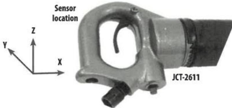
Figure C3 – Equipment handle image with superimposed coordinate axes.
